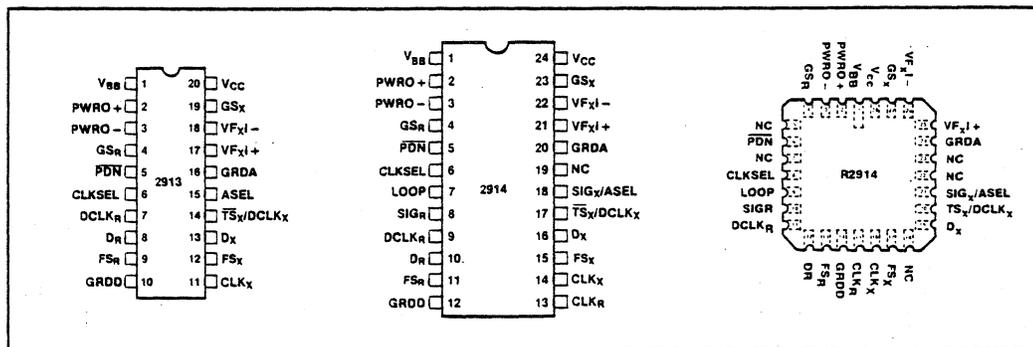
Figure 1. Pin Configurations
